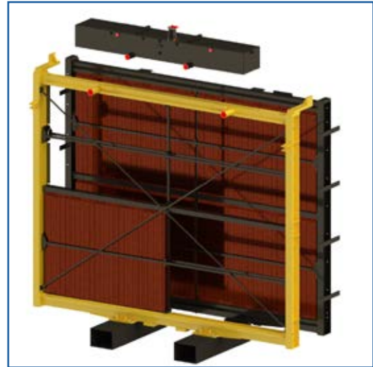
KOMATSU 960E-1/2 COOLING PACK AUTOCAD EXPLODED RENDERING
